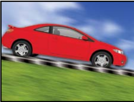
(a) On a low, downhill slope, use the third or the second gear.
