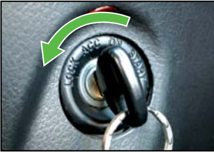
(a) Switch off the engine and withdraw the ignition key;
