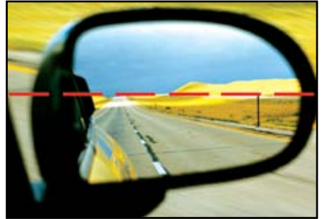
(b) Adjust the side mirror until the horizon is slightly above the centre line. Part of the body of your vehicle should be seen in the mirror.
