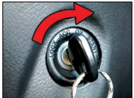
(d) Depress the accelerator pedal slightly and re-start the engine.
