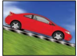
(c) Use the 1st gear and the footbrake together When the slope is short and steep
