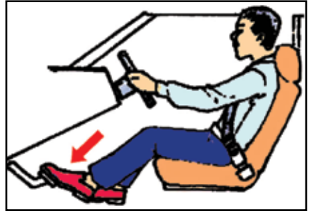
(b) Adjust your seat so that your left leg is almost straightened when the clutch pedal is fully depressed.
